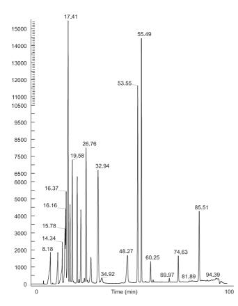
FIGURE 1. An HPLC chromatogram showing separation of twenty two standard phenolic compounds.
